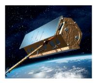
Atlas InSAR is Sixense's Interferometric Synthetic Aperture Radar (InSAR) solution to measure ground deformation and structure stability from space with millimetric precision.
