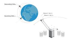
Radar interferometry is a Satellite remote sensing technique which is capable of measuring millimetric motion of terrain over wide areas.
